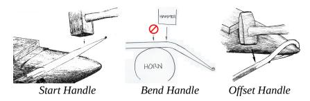
Quench the tip to protect it and form the handle over the anvil horn, curling the opposite direction. Curl the handle all the way around, then offset it to the centerline.
