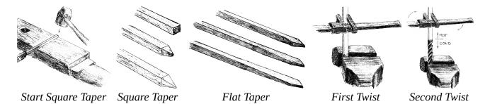
Twist the center section of the bar, above the flat taper. Add as many twists as wanted, quenching the twisted part when adding another twist. Leave the last 8 inches / 20 cm untwisted. Correct sideways bends with a wooden mallet on a wooden stump.
